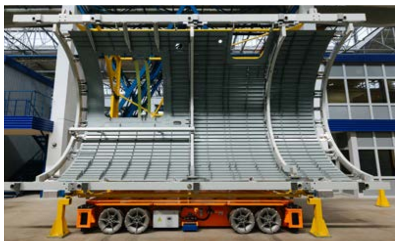
MS-21 aircraft fuselage panel at new assembly line station
