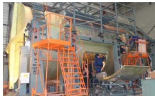
Fuselage assembly of MS-21 prototype aircraft
